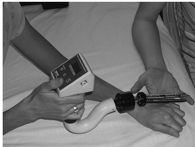
FIGURE 1. Rotterdam Intrinsic Hand Myometer used for the 5th-digit abduction strength test.
